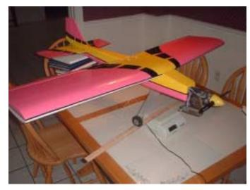
The weight of the main gear plus the ruler was 4 lbs 6.2 oz. The weight of the ruler alone was 1.5 oz. This would make the weight of the aircraft under its own gear equal to 4 lbs 4.7 oz.
