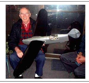
Ralph Snow completed this plane recently. It is an old time free flight called the Lancer. It was originally sized for a 30" wing span. Ralph enlarged the model to have a 50" wing span. It has a speed 40 with a 3:1 gear driven prop. It has 3 channels with rudder, elevator, and throttle. It will be powered with a 3 cell lithium polymer batter at 1500 MAH.
